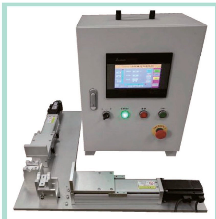
FIGURE 2 : Sclerosing foam preparartion machine.
