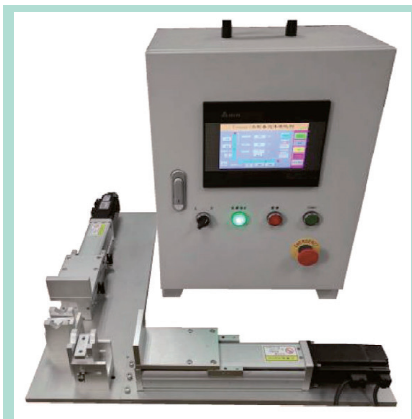
FIGURE 2 : Sclerosing foam preparartion machine.
