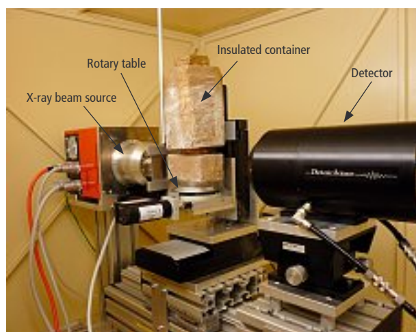
FIGURE 1 : The acquisition set-up at the Tomolab facility of Elettra (Trieste, Italy).
