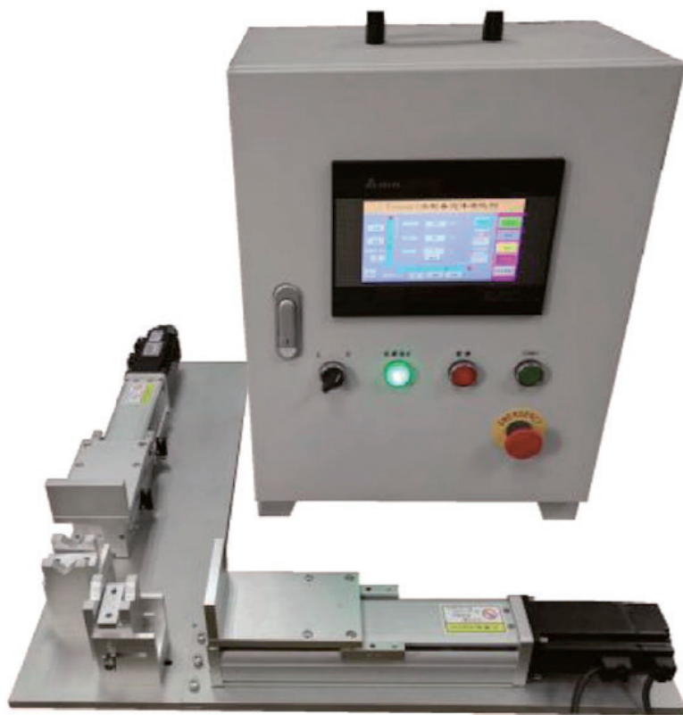
FIGURE 2 : Sclerosing foam preparartion machine.
